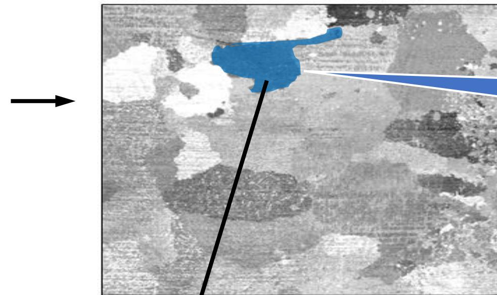
Crystal orientation in cold rolled steel
