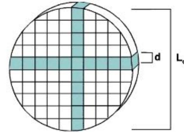
For a sphere a column height distribution is observed for any given  $hkl$ .  $L_{\text{vol}}$  is not identical with the diameter of the sphere, but can be derived from the known crystallite shape:  $L_0 = 4 L_{\text{vol}} / 3$  (Wilson, A.J.C. X-ray Optics, 1949)
