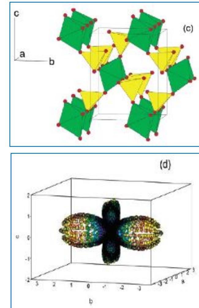
Spherical harmonics function used to model lattice strain in b-direction
