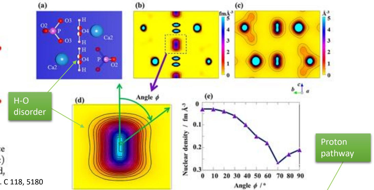
Figure 9. Refined structure with equi-density surface of difference bond valence sum (DBVS) at  $\pm 0.2$  v. u. at (a) 298, (b) 673, and (c) 923 K. Arrows indicate the bottleneck for the proton diffusion. Red,
