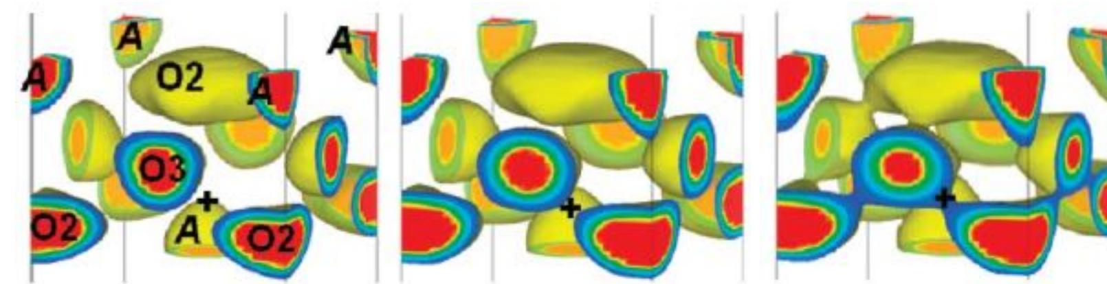
Equinuclear density surface at 0.05 fmÅ<sup>-3</sup> and nuclear density distribution on the (100) planes of (PLNCG) at different temperatures, which indicates the diffusional pathway of oxide ions in the crystal lattice of PLNCG.
