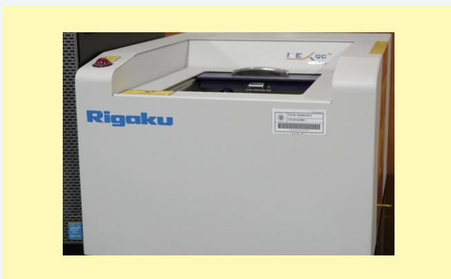
Gambar. Instrumen XRF NEX QC+ Rigaku
