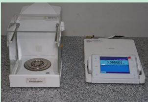
Gambar. Timbangan mikro resolusi 0,000001 gram
