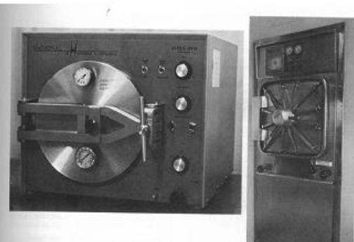
Fig. 4.3. Autoclaves. a. Bench-top model. b. Large, recumbent model. Both types now require that the pressure vessel cannot be opened until a safety pressure-release valve releases a safety lock, indicating a fall in pressure and temperature to a safe level.
