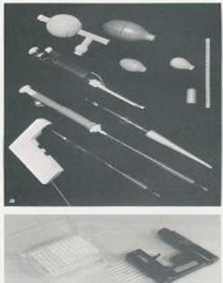
Fig. 4.10. *A*. Pipetting aids. Tip in bottom; various plastic bulb and bulb with inlet and outlet valves; Gilson and Kern-pipette micropipettes (take special plastic tips); Becton-Dickinson (standard pipettes); (see also Figs. 4.12, 5.3, and 5.6). *B*. Cetac multitipped pipette for loading microtiter plates.
