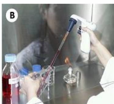
**Figure 5:** A: The vacuum pump with a 'trapping flask' protection. B: Glass or plastic pipettes with some form of suction aid are practical for transferring larger volumes.
